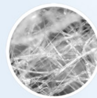
Magnified at 300x Non-HEPA Media Two Layers
